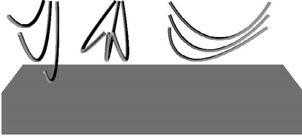
Figure 2: Suspended rope. Left to right : rest shapes for various end positions; swing side to side; sway back and forth.
